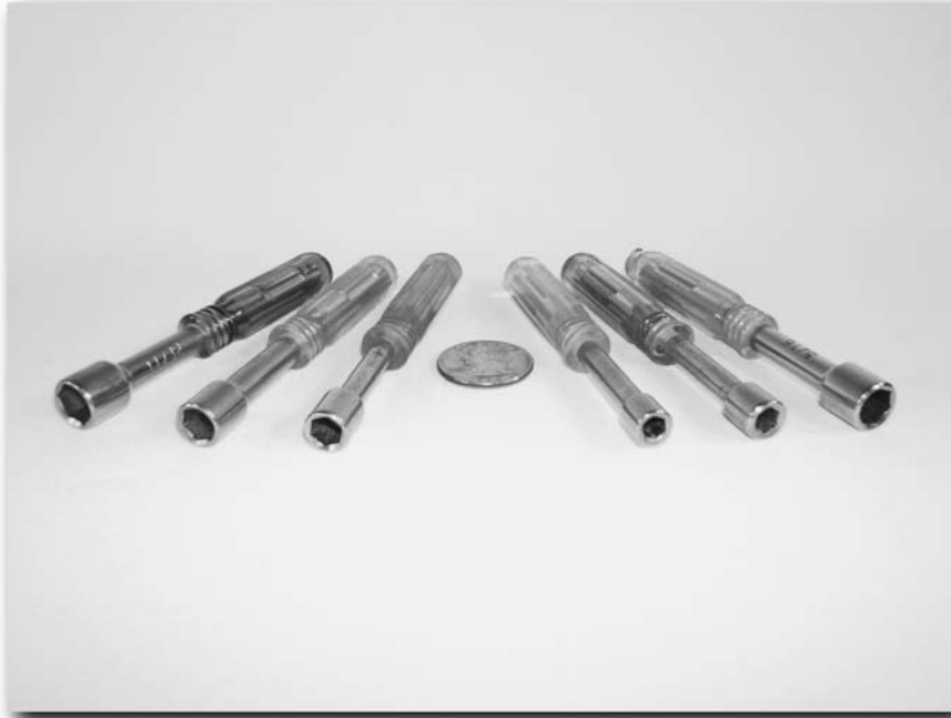
FIGURE 5-7: Socket drivers with hollow shafts
