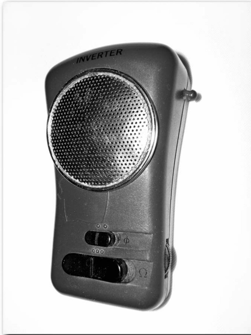
FIGURE 25-1: The Inverter (with internal mercury switch)
