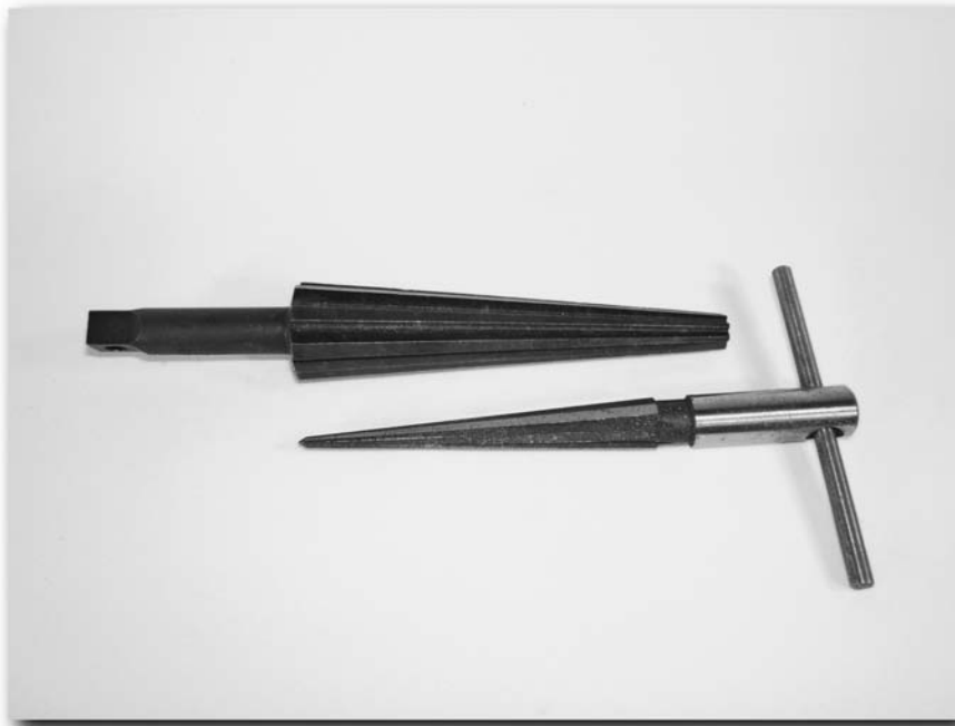
FIGURE 5-10: Tapered hand bore set
