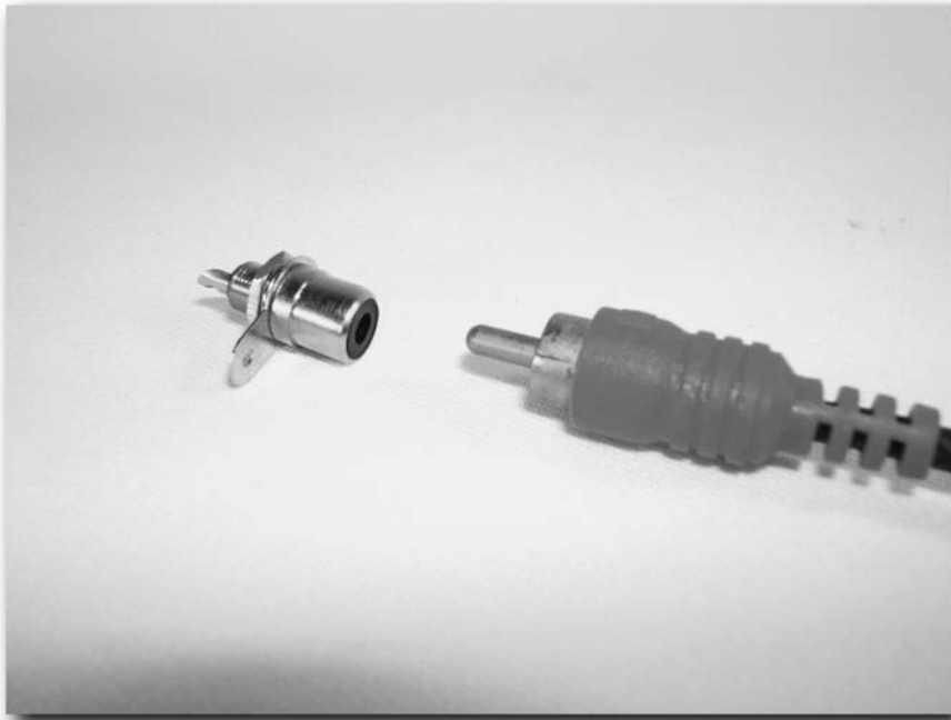
FIGURE 6-25: RCA jack and plug
