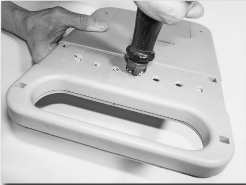
FIGURE 10-9: Use a de-burrer to smooth hole edges.
