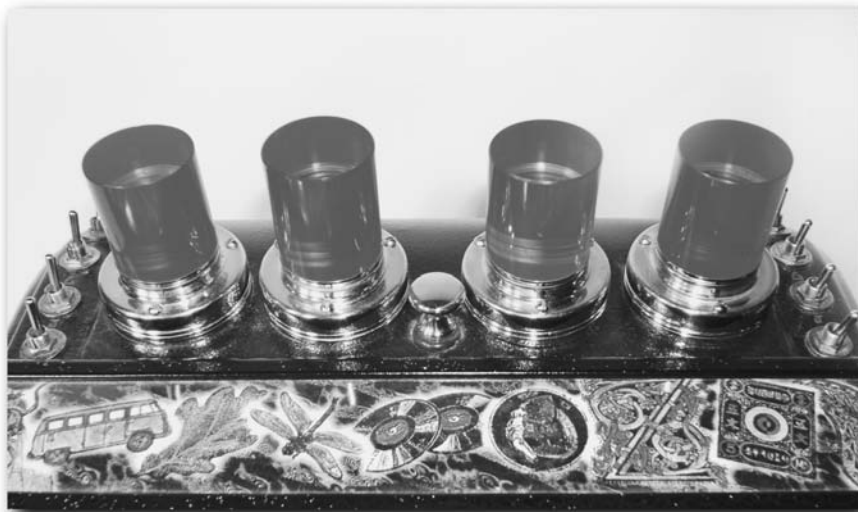
FIGURE 12-16: Light pipes on the Dworkian Register
