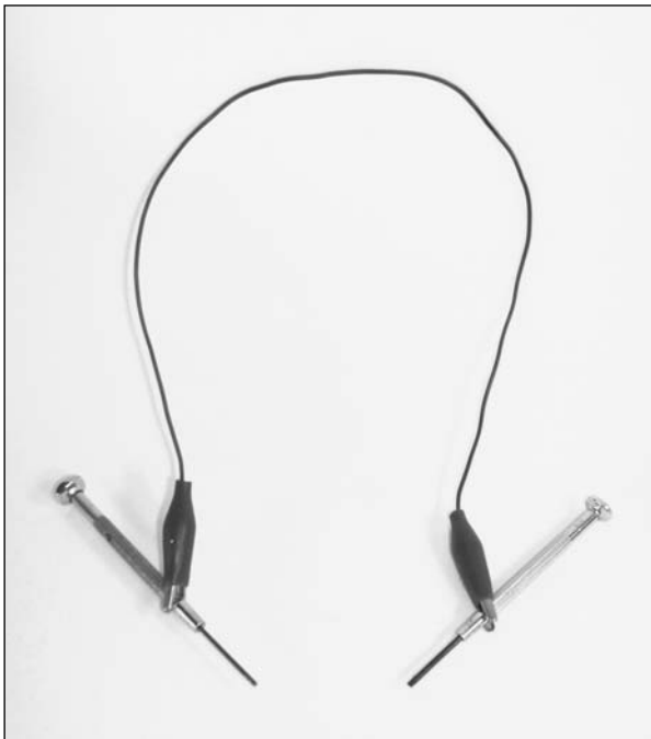
FIGURE 9-8: Alligator lead clipped to two small screwdrivers
