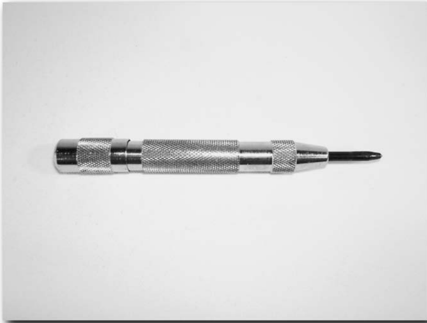
FIGURE 10-6: Use a center punch for locating holes to be drilled in metal.
